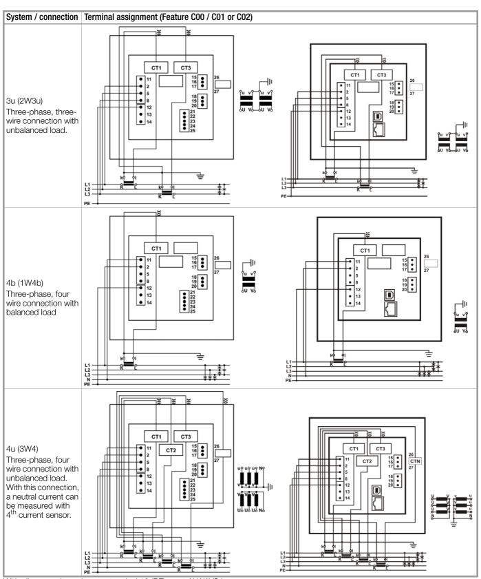
With all connection schemes, terminal 12 (PE) must ALWAYS be connected.
